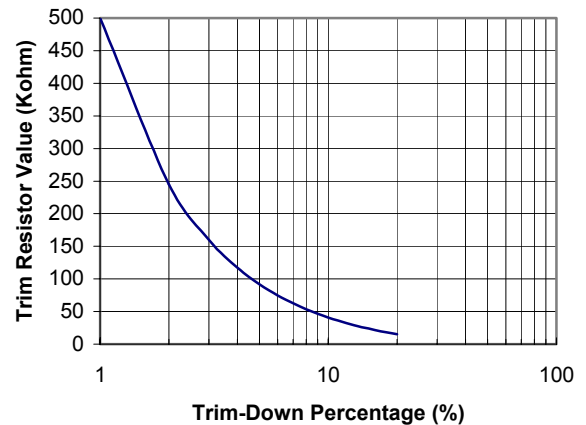
Fig. 18 Trim-Down Resistor Selection
