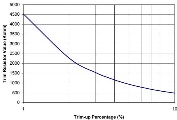
Fig. 19 Trim-Up Resistor Selection
